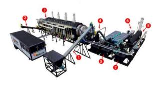
In addition to that, the facility is also going to have a thermal desorption unit of its own. This particular unit is going to be responsible for cutting materials that are heated to a temperature of as much as more than 640 degrees Fahrenheit. It is an important aspect of the plant and is meant for helping with vaporizing all the oil and water from cuttings.
